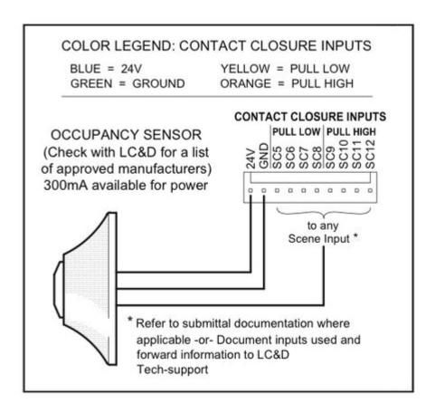
If more than one Occupancy Sensor is being used, the sensors can be wired in parallel if controlling the same lighting zone. If sensors are controlling different lighting zones then use different scene inputs.
