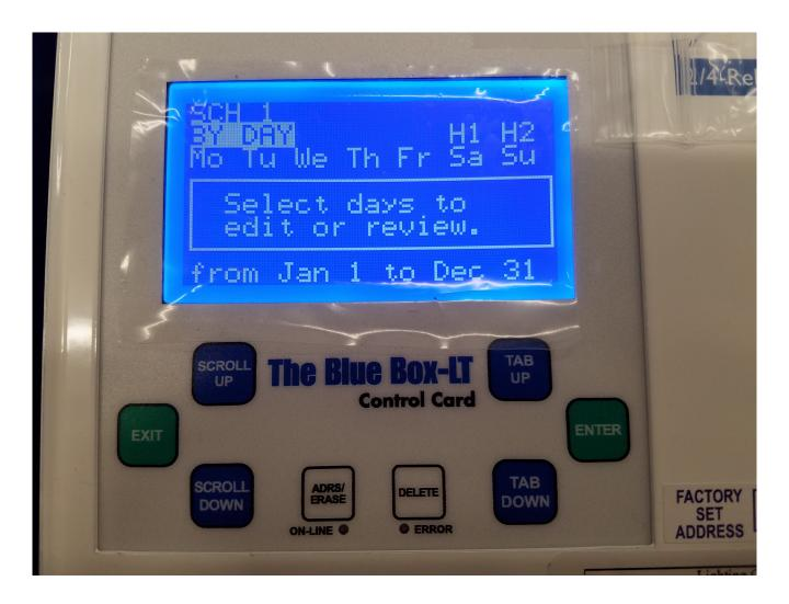
A BY DAY schedule is used when different on and off times are needed for different days of the week. Press ENTER on any day of the week to change the on and off times for that day. BY DAY schedules can also be set up to run within a certain range of dates. This range can be adjusted at the bottom of the BY DAY schedule screen.
