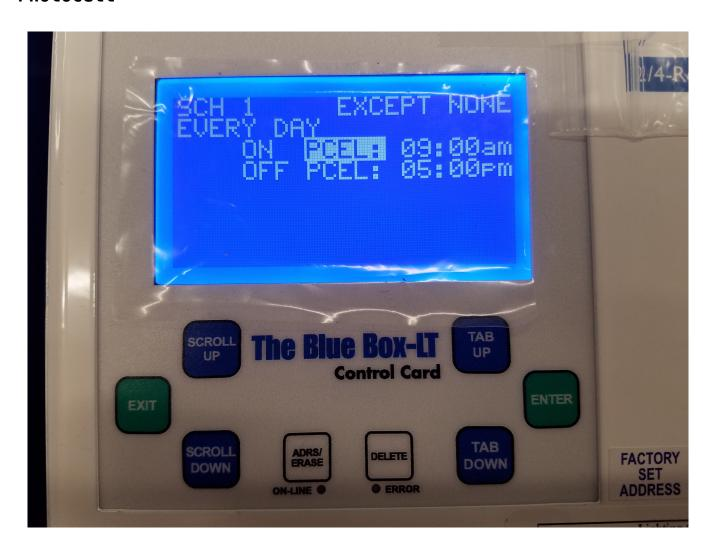
When a schedule displays ON PCEL or OFF PCEL, it is switching based on a photocell. The ON PCEL time indicates what time the onboard photocell, in a BlueBox, is going to start controlling the group. At the OFF TIME, the lights sweep off, and the photocell relinquishes control of the group. If you have the word PCEL selected, and you press ENTER, you will see this screen:
