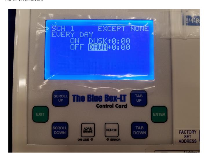
When a schedule displays ON DUSK, ON DAWN, OFF DUSK, OR OFF DAWN, it is switching its group according to an astronomical clock. Using this method, the controller will use the longitude and latitude entered in its SYSTEM OPTIONS, to calculate the DUSK and DAWN times. DAWN indicates the time that the sun rises. The times that the controller calculates dusk and dawn to be, will flash periodically on the start screen of the system controller.
