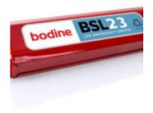
Bodine BSL23C LED Emergency Driver. The BSL23C emergency LED driver works in conjunction with an AC LED driver that has an output current not to exceed 1.5 A, convert new or existing LED fixtures into emergency lighting. The emergency driver consists of a high-temperature nickel-cadmium battery, charger and electronic circuitry in one compact red case.
