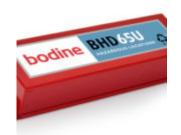
Bodine BHD65U Hazardous Location Emergency Driver Hazardous LocationsOne- or Two-Lamp Illumination Universal Input (120 through 277). The BHD65U Universal Input emergency ballast works in conjunction with an AC ballast to convert fluorescent fixtures into emergency lighting. The emergency ballast handles a wide range of input voltages and frequencies and consists of a hightemperature nickel cadmium battery, charger, hermetically sealed relays and electronic circuitry in one compact red case.
