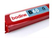
Bodine B60 Emergency Ballast. The B60 emergency ballast works in conjunction with an AC ballast to convert new or existing fluorescent fixtures into emergency lighting. The emergency ballast consists of a high-temperature nickel-cadmium battery, charger and electronic circuitry in one compact red case. For damp locations; two-lamp emergency illumination; end-of-lamp-life compatible.
