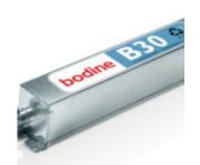
Bodine B30 Emergency Ballast. Works in conjunction with an AC ballast to convert new or existing fluorescent fixtures into emergency lighting. The emergency ballast consists of a nickel-cadmium battery, charger and electronic circuitry in one case. Can be used with most 17-215~W~(2'-8')~T5, T8, T9, T10 or T12 fluorescent lamps without integral starters
