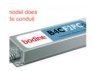
Bodine B4CF2P Emergency Ballast. The B4CF2P emergency ballast works in conjunction with an AC ballast to convert new or existing fluorescent fixtures into emergency lighting. The emergency lighting equipment consists of a high-temperature nickel-cadmium battery, charger and electronic circuitry in one compact case. Specification grade; one- or two- lamp parallel operation emergency illumination.
