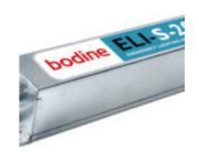
Bodine ELI-S-20 Emergency Lighting Inverter. Sinusoidal (Sine Wave) Output 20 or 25 Watts Power Auto Select 120 or 277 VAC Code-Compliant 90-Minute Runtime.
