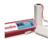
Bodine BSL722 LED Emergency Driver 23.1 Watts output power. The BSL722 emergency LED driver works in conjunction with an AC LED driver to convert new LED fixtures into emergency lighting. The emergency driver unit consists of a battery charger and electronic circuitry in one compact case.
