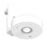
This is the dual technology occupancy sensor fixture mount w/height adjuster. The Lightcloud Sensor is a dual-technology motion detector that can switch and dim both local and remote circuits. It monitors power consumption, and can send an alert if power is lost. The Sensor is available for both standard and high bay applications, each with the option of surface or fixture mounting.
