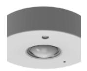
This is the dual technology lightcloud sensor ceiling mount. The Lightcloud Sensor is a dual-technology motion detector that can switch and dim both local and remote circuits. It monitors power consumption, and can send an alert if power is lost. The Sensor is available for both standard and high bay applications, each with the option of surface or fixture mounting.
