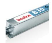
Bodine B30 Emergency Ballast. Works in conjunction with an AC ballast to convert new or existing fluorescent fixtures into emergency lighting. The emergency ballast consists of a nickel-cadmium battery, charger and electronic circuitry in one case. Can be used with most 17 – 215 W (2' – 8') T5, T8, T9, T10 or T12 fluorescent lamps without integral starters AC/DC Output for T5 or T8 lamps suitable for one- or two-lamp Operation for up to 3500 Lumen Output. Universal Input 120V through 277V.
