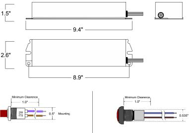
BSL36Cold ships with a 2-wire illuminated test switch/charging indicator light.
