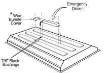
If the application requires the product to be mounted on top of the luminare please use wire bundle cover kit (RMC-60). Please note, the RMC-60 kit contains enough parts to install two products.
